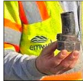
BROKEN PIPE: (Left) An EMWD worker holds a section of Orangeburg piping that broke under Via Playa del Rey.
